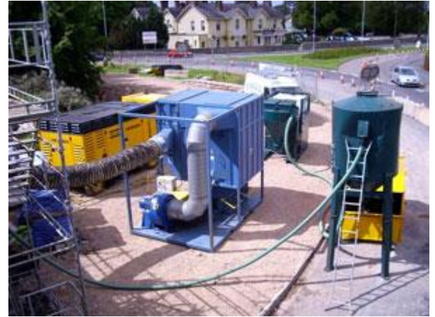
6000 cfm Dust Extractor (left) and shown on Site (right) with Hopper and Abrasive Recovery
